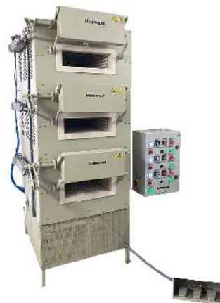
HCV42/13 3CX Heat treatment Furnace Max. Temperature 1300°C 3 chamber in 1
