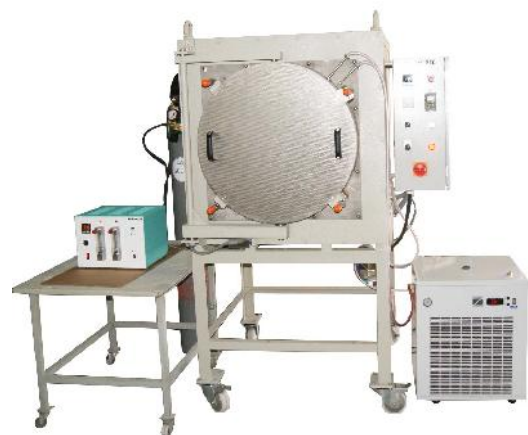
HCV CCH Series Retort furnaces Temp. up to 1150°C Heat treatment under controlled atmosphere
