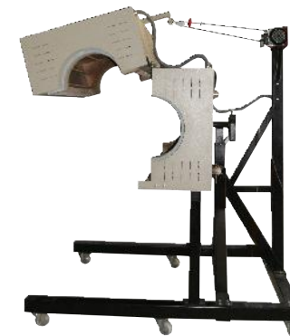
TR15XL Vertical and Horizontal operation Automatic Opening Beams testings
