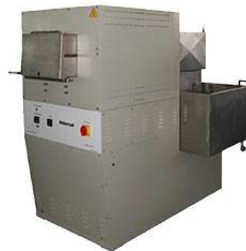
ATF Series (Static) Fast cooling Temp. up to 1150°C Tempering and annealing applications
