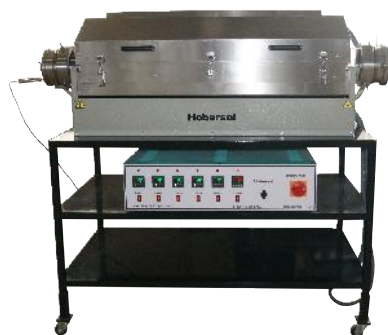
ST SP series Split tube furnaces Max. Temperature 1200°C Heated length: 200 to 2000mm
